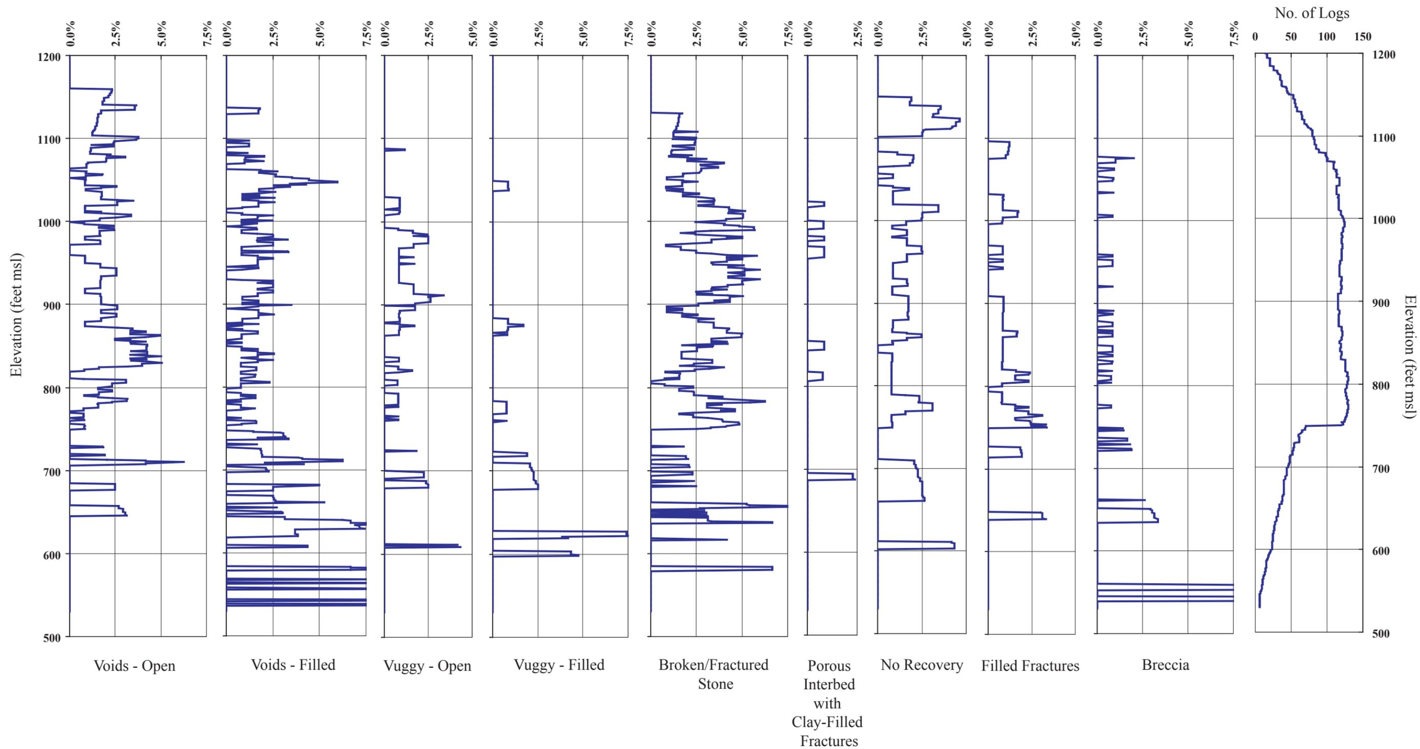
Elevation-Averaged Occurrence of Voids and Enhanced Porosity Encountered by Quarry Borings (215 total logs)
